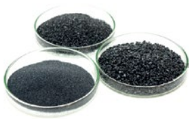
SILICON CARBIDE (SiC) POWDER Mixed into paste & extruded
