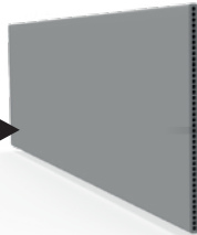
SUBSTRATE Extrusion fired @ >2,200 °C to bond SiC grains
